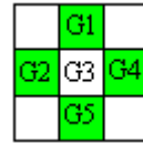
Fig 6. Edge-directional interpolation. G1, G2, G4, G5 – given green pixels, G3 – interpolated green pixel.
