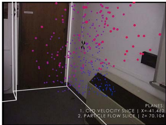
Figure 14: Registration of virtual white lines and graphical objects in actual-space, as seen from HMD.
