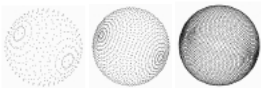
Figure 5: Sampling of the surrounding sphere to determine initial set of camera positions.
