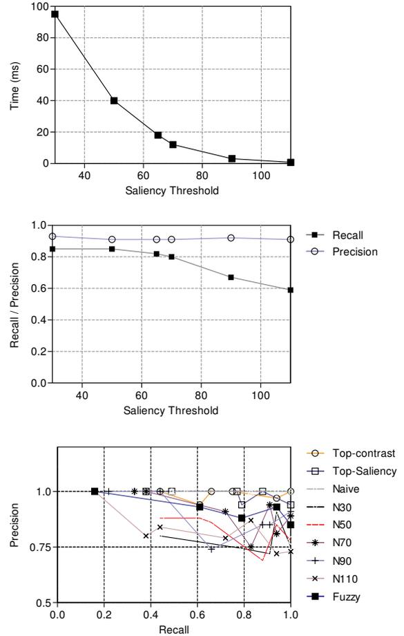
**Figure 6:** Evaluation results. Upper plot: dependency of average matching time on saliency threshold. Middle plot: dependency of accuracy metrics on saliency threshold. Lower plot: recall-precision graphs.
